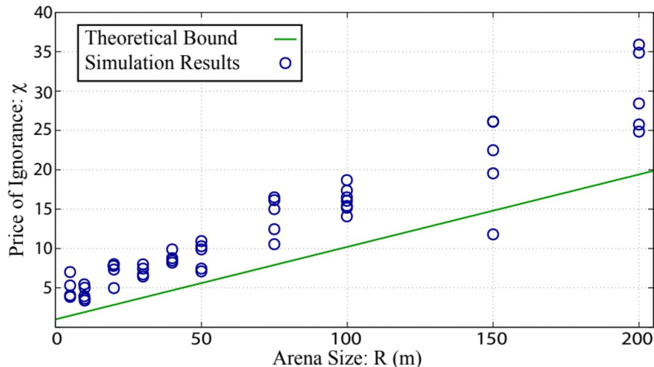
Argos Robot Simulator [7], 5 trials per arena size, 10 robots per trial, 4 clusters of 64. Collisions.
