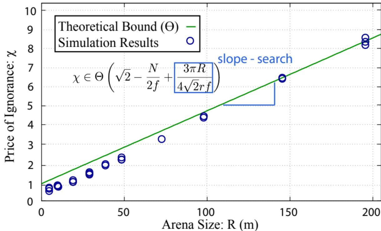
Argos Robot Simulator [7], 5 trials per arena size, 10 robots per trial, 4 clusters of 64.
